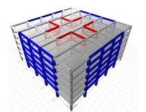
Image 1 Schematic representation of a complete model. SFRS as SCBF (in red interior) and OMF (in blue exterior) as a back-up system
