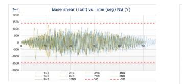
Image 6. Max shear forces at the base for all ground motions, Y sense (top), X sense (bottom)
