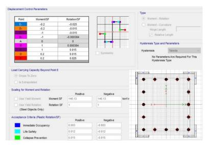
Image 5. Plastic hinge parameters of a column of the SFRS
