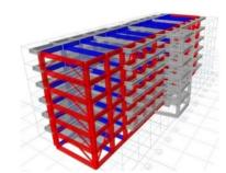
Image 2 Analysis models for the project. Complete system, (in red interior) and OMF (in blue exterior) as a back-up system
