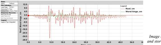
Image 8 Displacements at the roof and storey 2, ground motion 6NS (Y)
